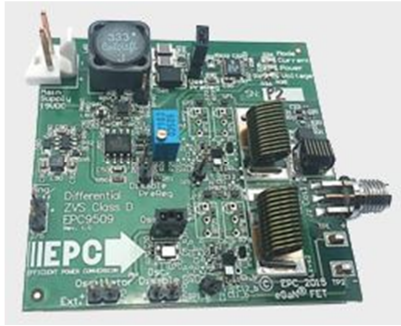
(그림 14) EPC9509(60V ZVS Class-D Amplifier Board for Wireless Power Transfer Systems)[20]
