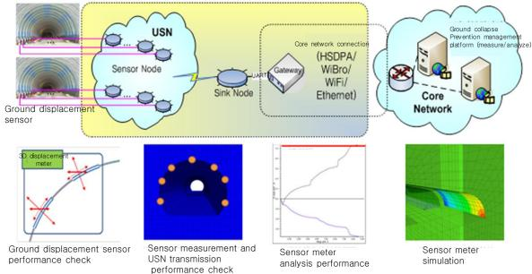
[Wireless sensor network based ground displacement remote transmission and data analysis system diagram]
