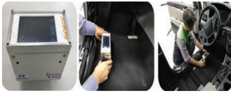
ETRI's portable water leak testing system to monitor the water-leaking failure in the car manufacturing
