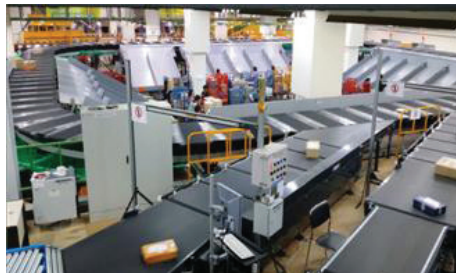
A parcel sorter developed by ETRI operation at the Busan Postal Distribution Center
