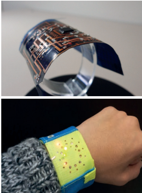
Copper fabric circuit board (top) and fabric watch (bottom)
