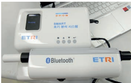
Lung cancer diagnose system by analyzing exhaled breath components
