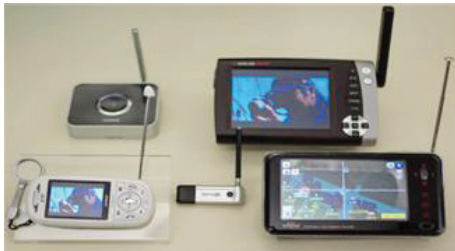
Terrestrial DMB receiving SoC and prototypes of DMB terminal
