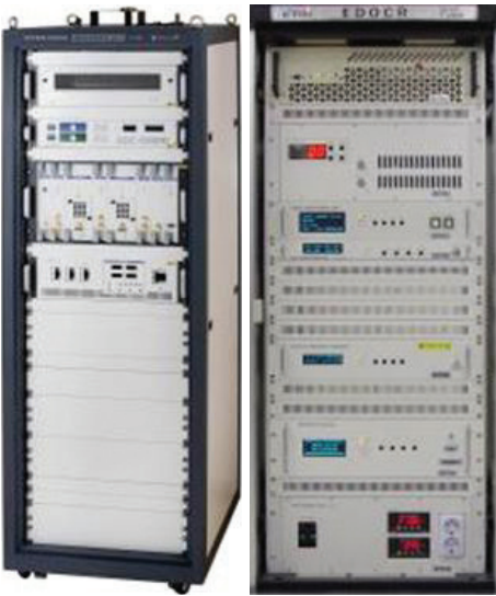
DTxR(Distributed Translator)(Left) and EDOCR(Equalization Digital On-Channel Repeater) (right)
