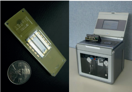
Cancer biomarker detection semiconductor biochip and reader for point-of-care diagnosis
